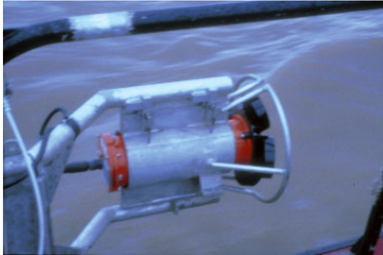
Figure 4.2. Acoustic Doppler Current Profiler (ADCP) mounted to the boat.
