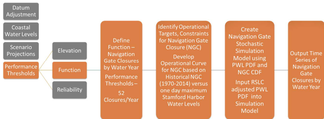
Figure 54 - Workflow for Function-Time series performance model (NGC/Water Year) for the Stamford Hurricane Barrier
