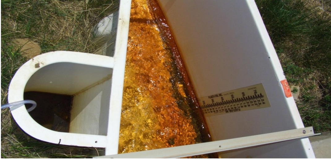
Figure C-35: Stage indicator and bubbler at CG-5 flume.
