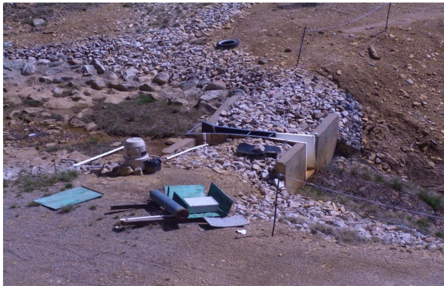
Figure C-6: CG-1 gauge in California Gulch. Flow from left to right. Tan colored container is auto-sampling unit.
