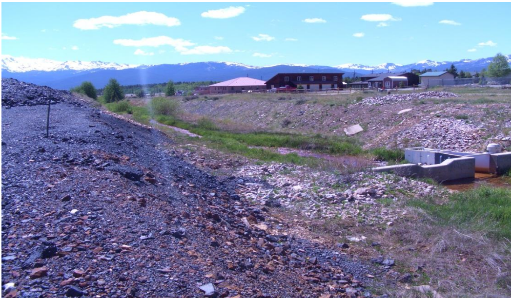
Figure C-24: View from left bank of California Gulch looking downstream beyond CG-4 gauge. Note high-flow notch in gauge weir.
