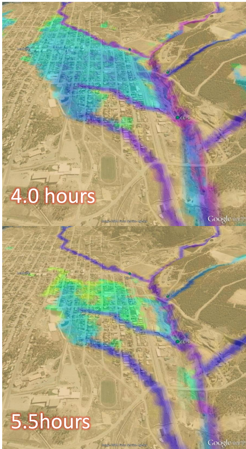
Figure 7.6: Close-up showing potential for interactive evaluation of flash-flood inundation using KML to interpret output from 100-year storm TREX model on Google Earth 3-D oblique imagery. Red text indicates number of hours after beginning of rainfall.
