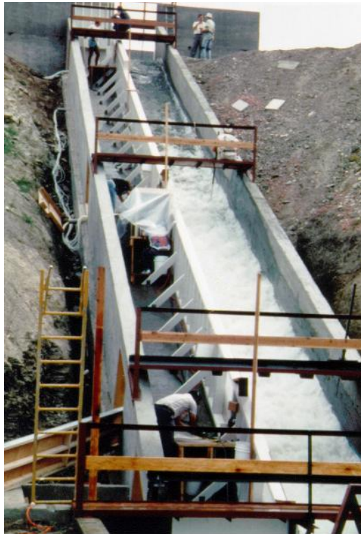
Figure 4.1 Physical model of the stepped spillway (Ward, 2002)
