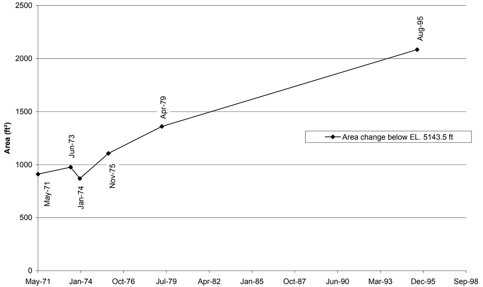
Fig. E-40. Change in cross section area with time at cross section CO-13.
