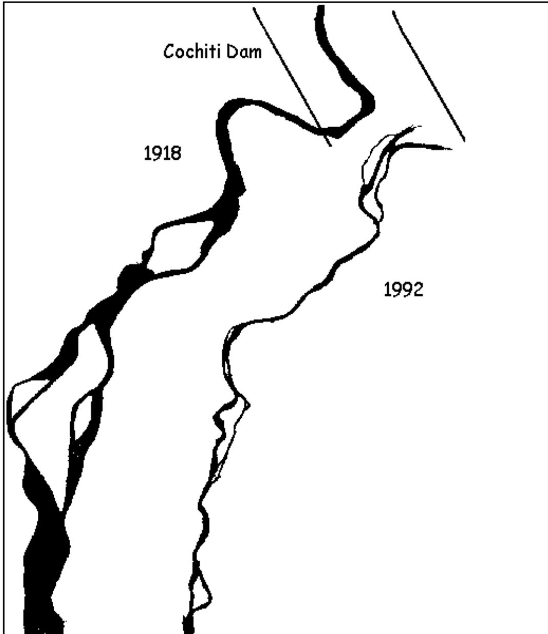
Fig. 2.2. Planform comparison below Cochiti Dam from 1918 to 1992.
