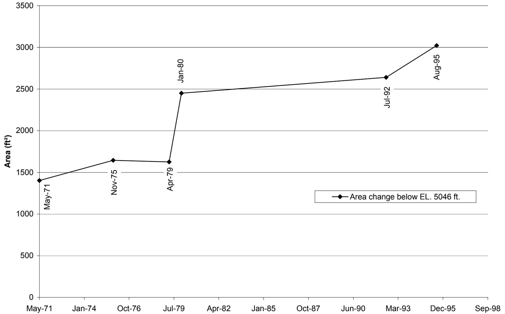
Fig. E-57. Change in cross section area with time at cross section CO-30.
