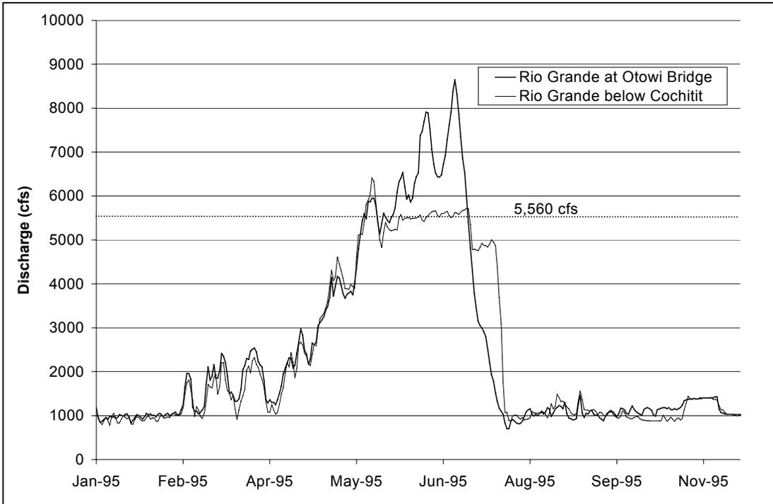
Fig. 3.5. 1995 flow hydrograph of Rio Grande at Otowi Bridge and Rio Grande below Cochiti Dam gaging stations.
