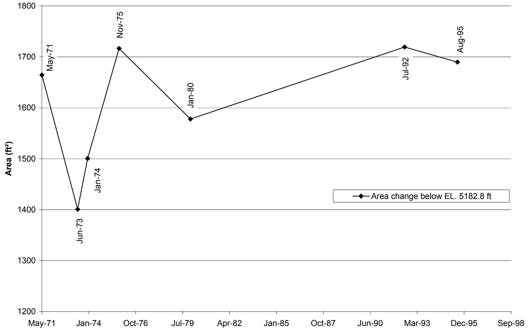
Fig. E-34. Change in cross section area with time at cross section CO-7.
