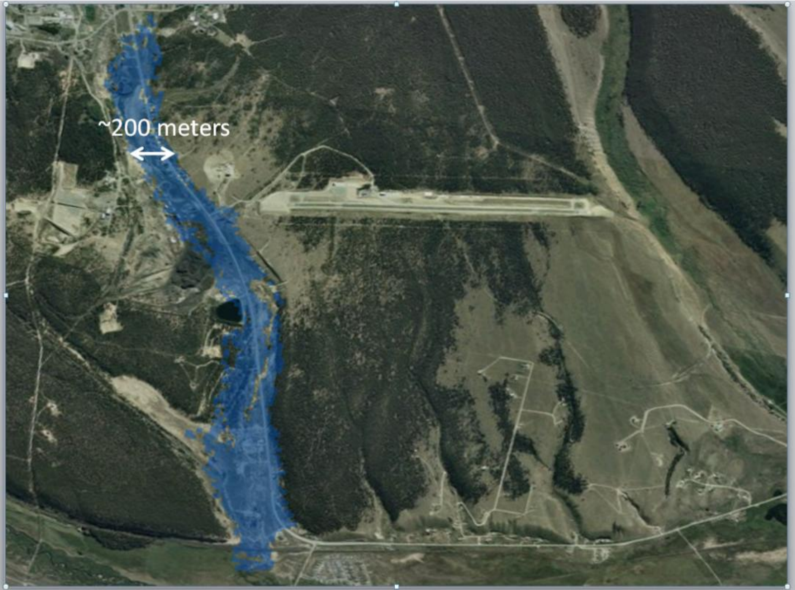
Figure 5.6: 4,000 m 3 /s point source floodplain inundation at 45 minutes after flood wave introduction, (depth \geq 1 meter)
