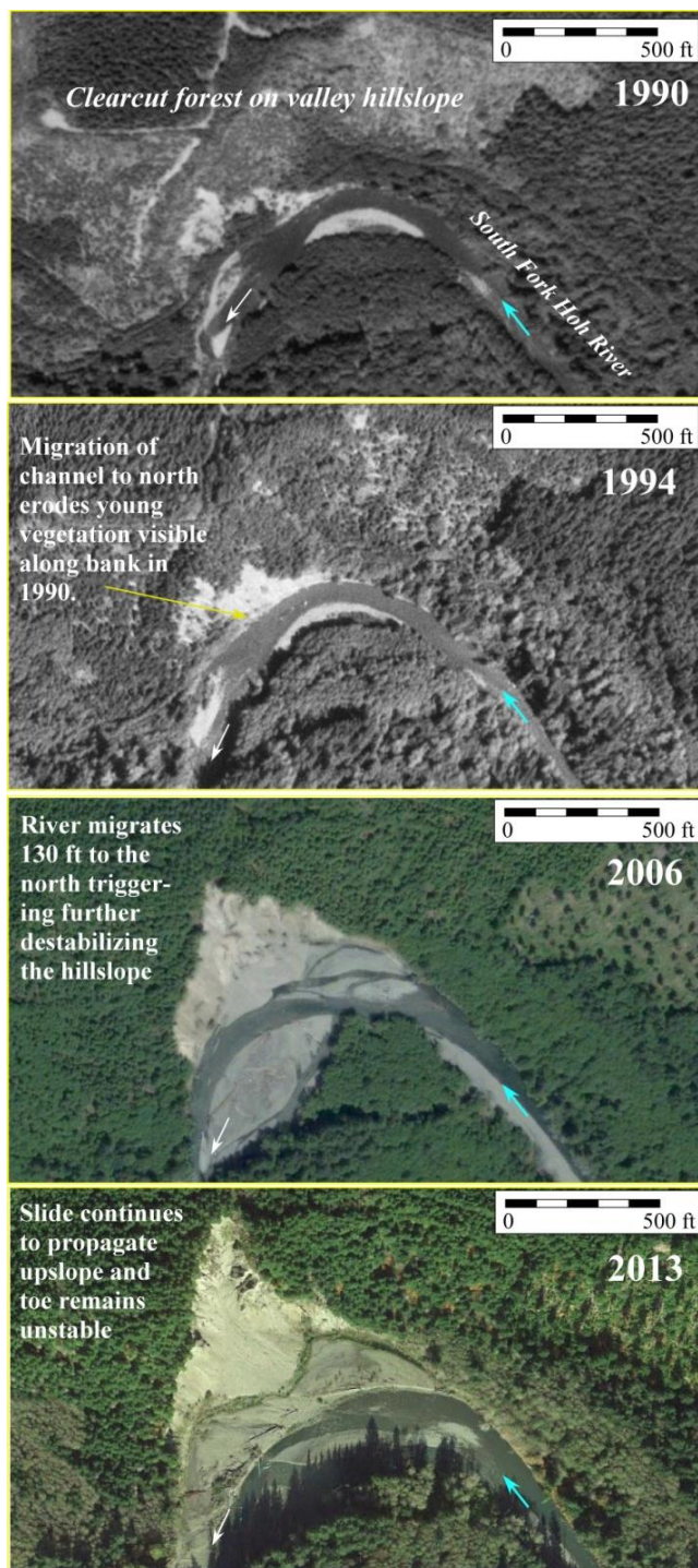
Figure 4-37. Clearing Mature Riparian Forests Eliminates Functional Wood Recruitment and Alters Processes and Channel Form
