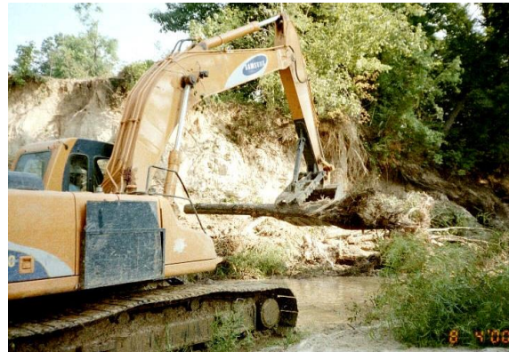
Figure 8-2. Equipment Useful for Handling Large Wood
