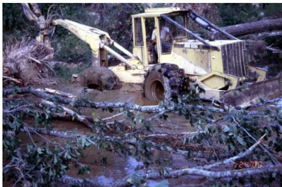
Figure 8-14. Log Skidder Mired in an Isolated Deposit of Highly Plastic Clay in a Stream Bed
