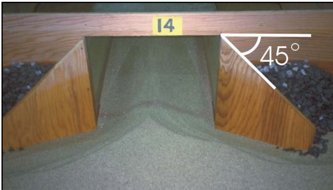
Figure 6.16. Rectangular model with wing walls (FHWA 2003a).
