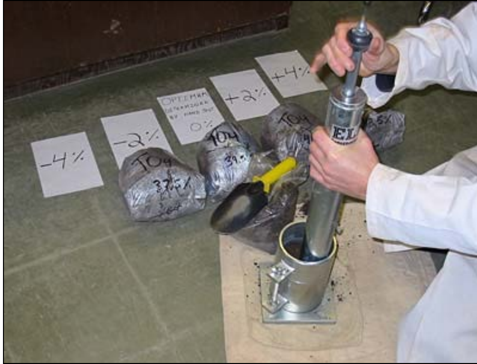
Figure 4.14. Standard laboratory compaction test (from the University of British Columbia web site).
