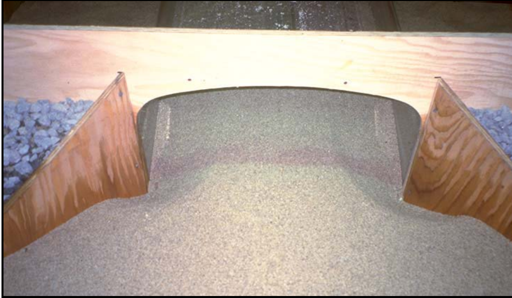
Figure 6.17. Arched model with wing walls (FHWA 2003a).
