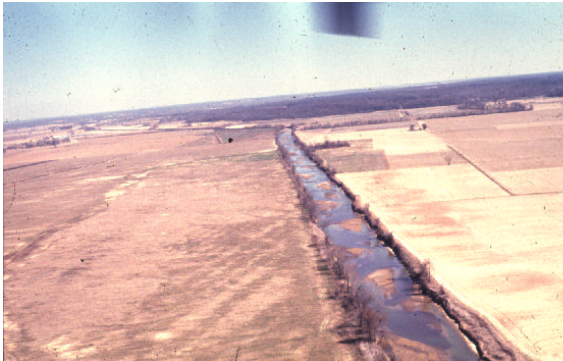
Figure 3.8 Typical Alternate Bar Pattern
