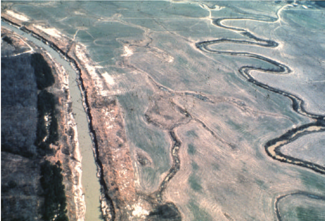
Figure 3.21 Channelized Stream and Abandoned Old Channel
