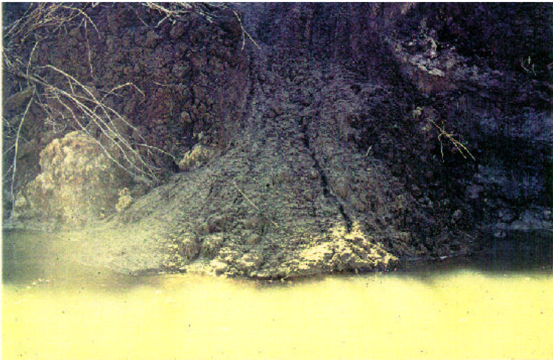
Figure 3.38 Wet Earth Flow
