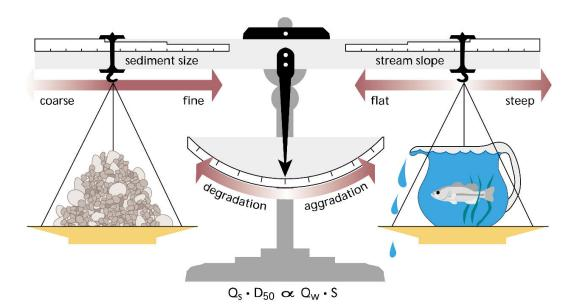
Figure 1.—Lane's channel stability balance describes how changes in sediment load, size, stream slope, discharge, and channel roughness determine whether a channel will aggrade or incise [7].
