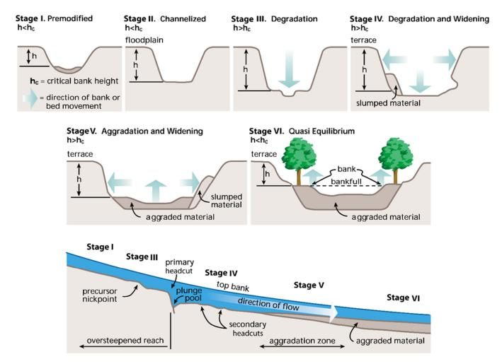
Figure 2.—Channel evolution model for incised channel response after a disturbance ([7], adapted from [11]).
