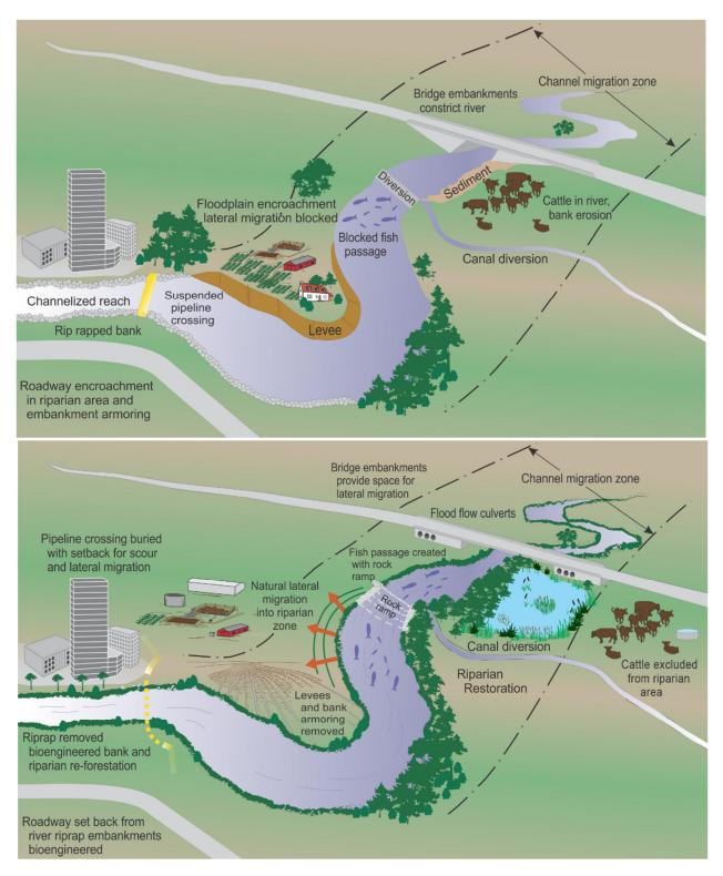
Figure 5.—Illustrations of riverine infrastructure with greater impacts to physical stream processes and ecosystems and greater exposure to riverine hazards (top) and more resilient and stream compatible infrastructure that permits a greater degree of channel movement supporting ecosystem processes (bottom).
