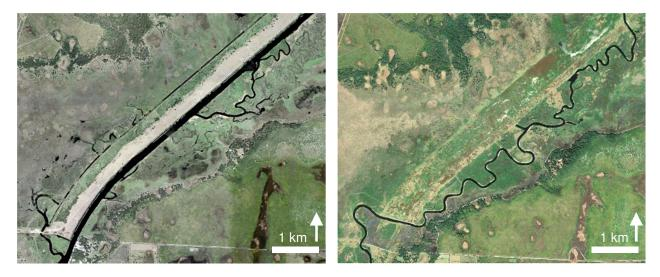
Figure 13.—Channelized reach of Kissimmee River (left) [77], and restored reach with meandering planform and channelized Reach Filled (Right) [78].
