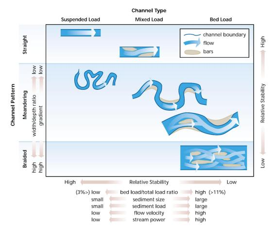
Figure 3.—Classification of channel type and pattern (planform) as a function of sediment size and load ([7] adapted from [11].
