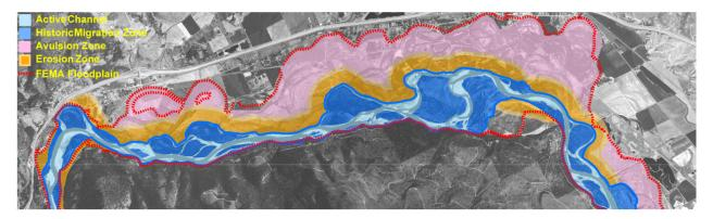
Figure 4.—Example of a channel migration zone study depicting the active channel (light blue), historic channel migration zone (dark blue), future erosion buffer (orange), potential channel avulsion zone (pink), and regulatory floodplain (dashed red line). Clark Fork River, Montana, Applied Geomorphology, Inc., DTM Consulting, Montana State Geographic Information Clearinghouse.
