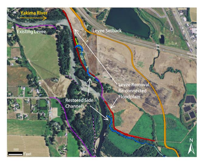
Figure 10.—An example of a proposed levee setback and side-channel rehabilitation project on the Yakima River, Washington. Hydrologic connection restored to western floodplain. Map courtesy of Robert Hilldale, Bureau of Reclamation. Setback alignment still under discussion.
