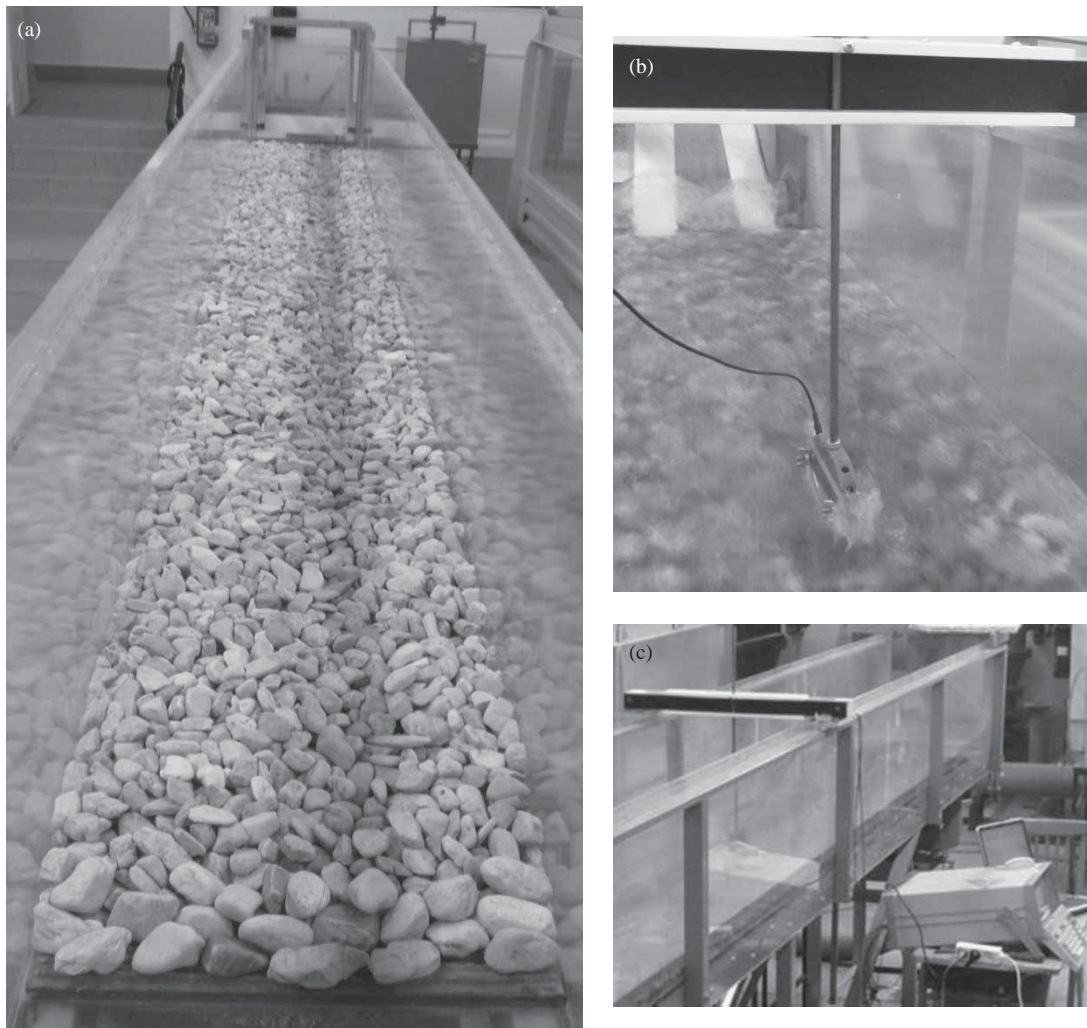
Figure 2 Experimental flume and velocity measurement technique
