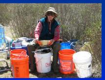
Washing samples to separate coarse organic material from bedload
