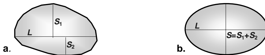
Fig. 4.13: Axes L , S_1 and S_2 fitted by computer into the outlined and digitized particle shape (a); Computer-fitted ellipsoidal reference particle shape for computation of particle volume (b). (Redrawn from Ibbeken and Schleyer (1986), by permission of John Wiley and Sons, Ltd.).
