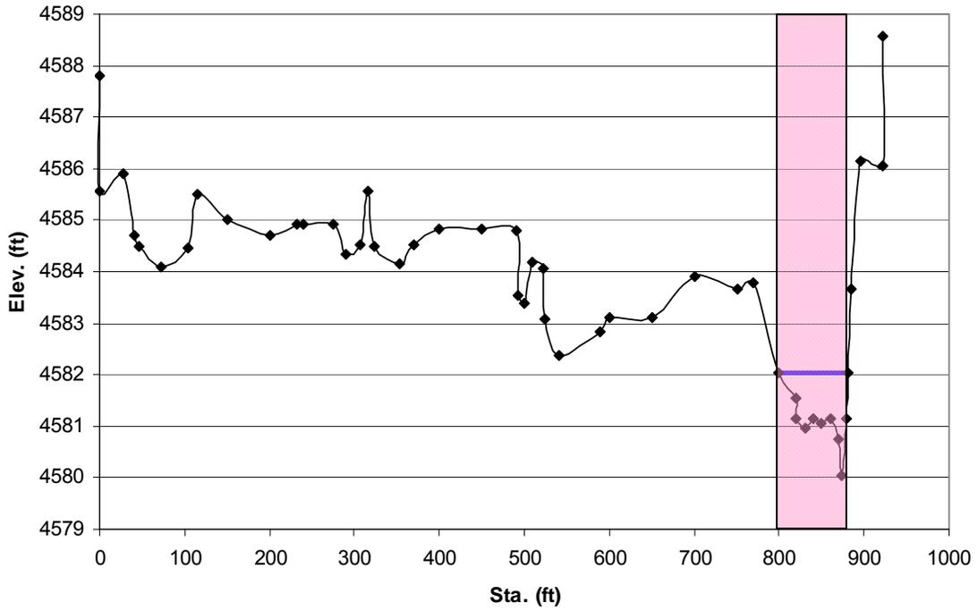
Figure E.4 Cross-section 1380 (surveyed 9/12/1990, Q = 70 cfs)
