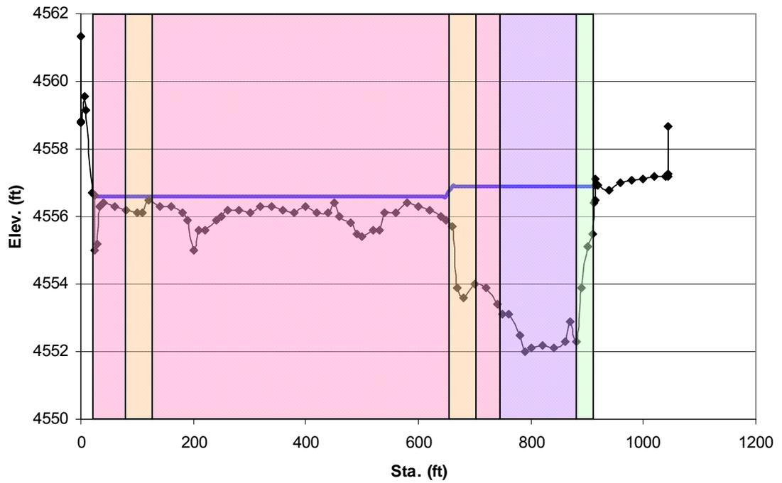
Figure E.7 Cross-section 1450 (surveyed 5/27/1993, Q = 5000 cfs)
