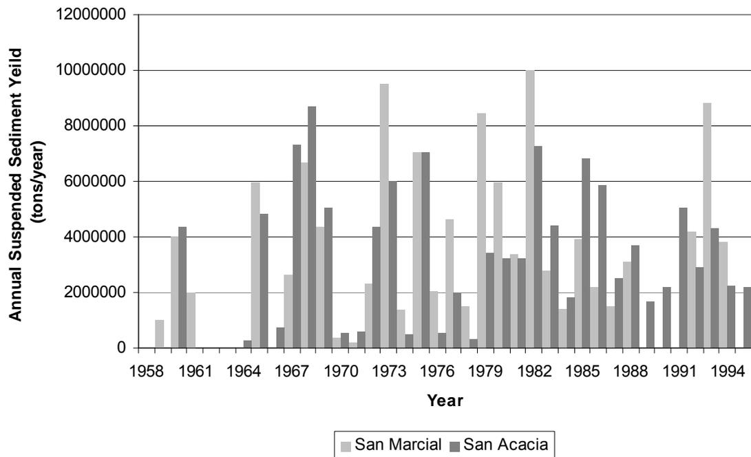
**Figure 2.6 Annual Suspended Sediment Yield at San Acacia and San Marcial Gauges**
