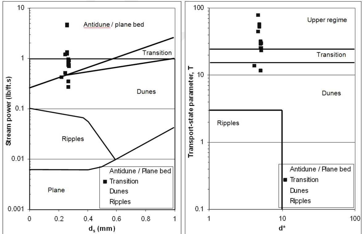
Figure 6.5 Observed transition bedforms plotted on graph from Simons and Richardson (L) and van Rijn (R) (after Julien 1998)
