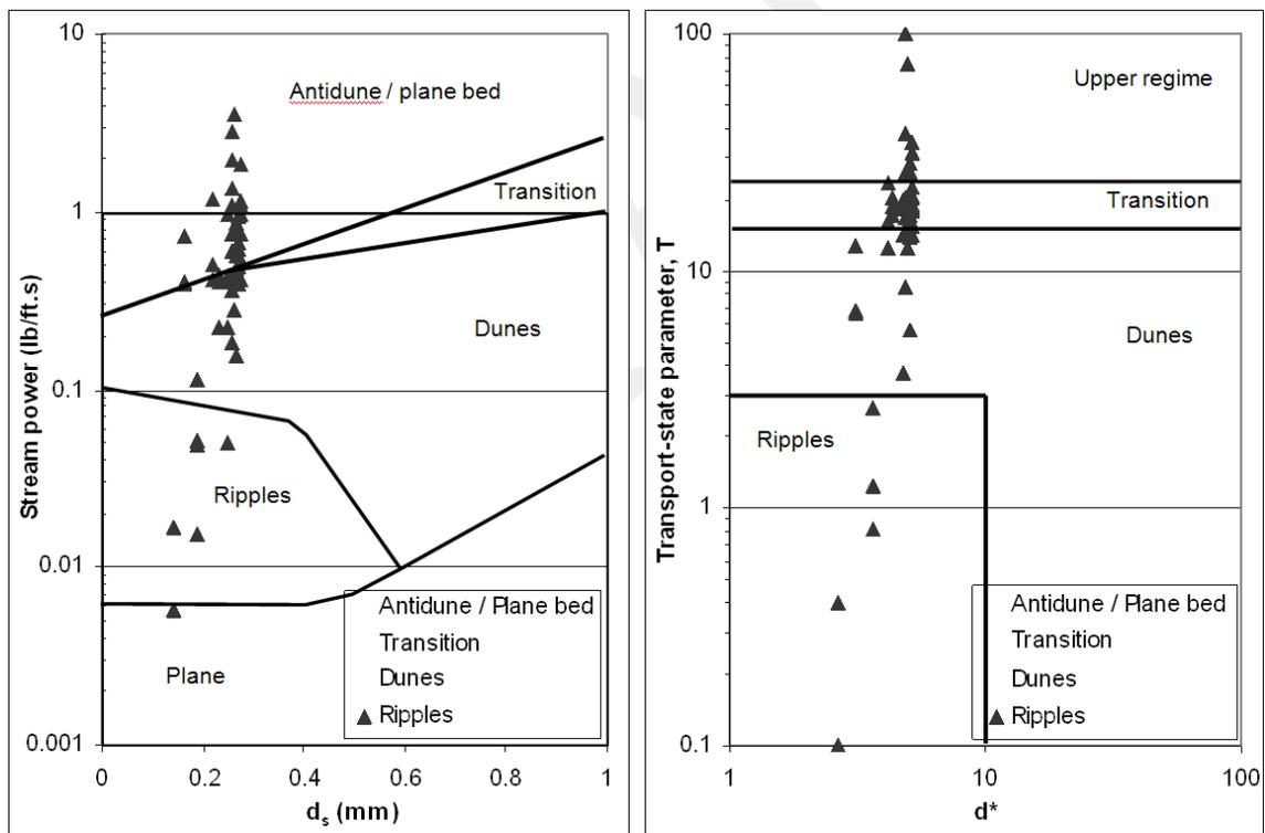
Figure 6.3 Observed ripples plotted on graphs from Simons and Richardson (L) and van Rijn (R) (after Julien 1998)
