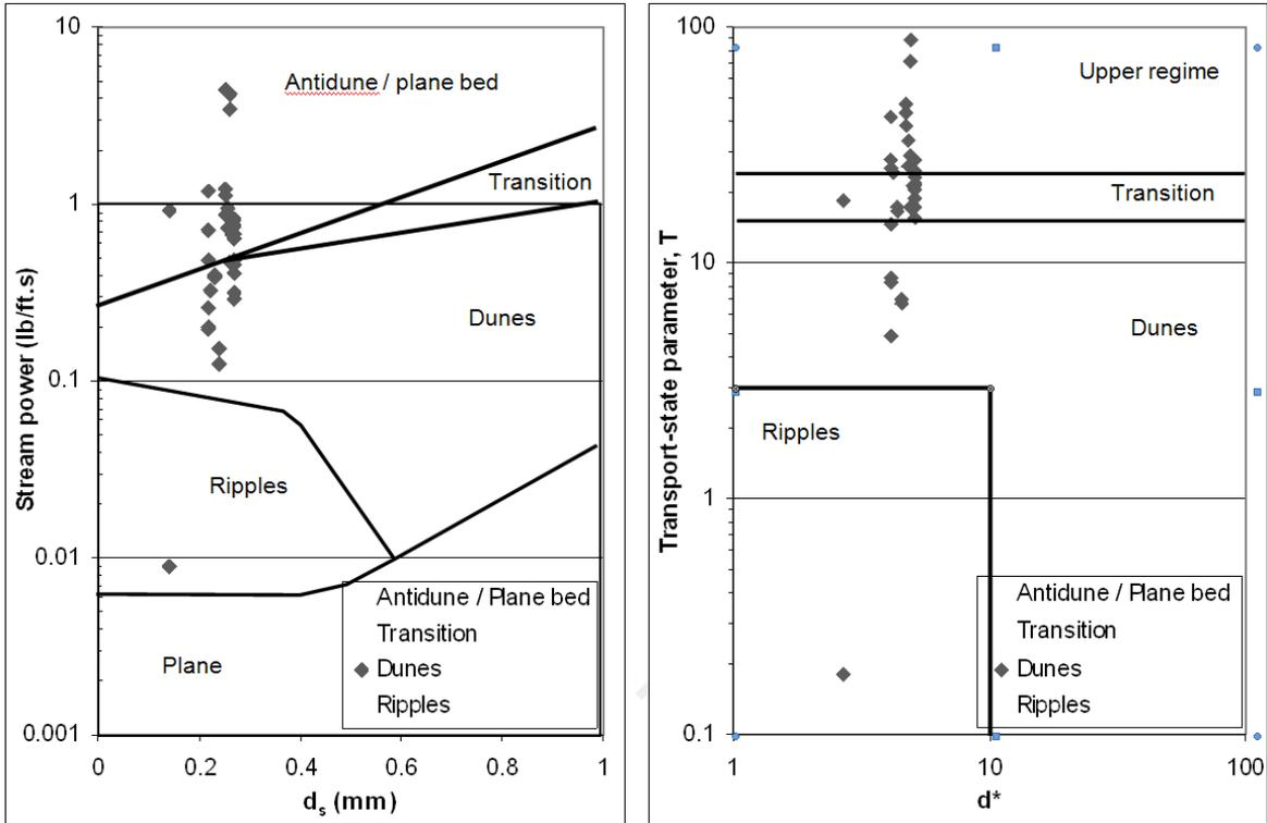
Figure 6.4 Observed dunes plotted on graph from Simons and Richardson (L) and van Rijn (R) (after Julien 1998)
