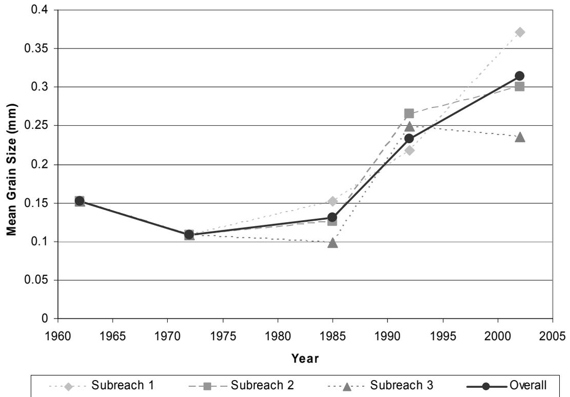
**Figure 3.16 Bed material mean grain size**
