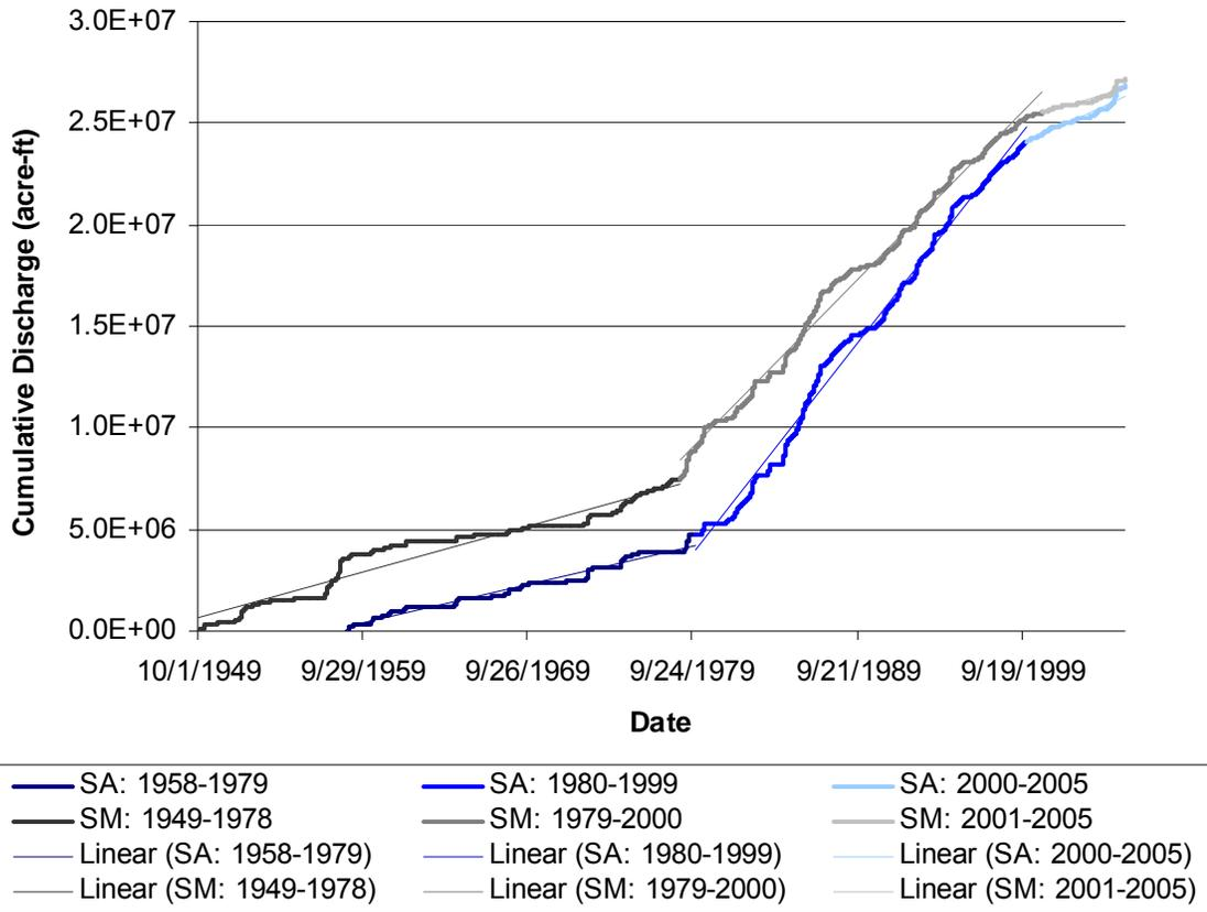
Figure 4.1 Water Discharge Single Mass Curve
