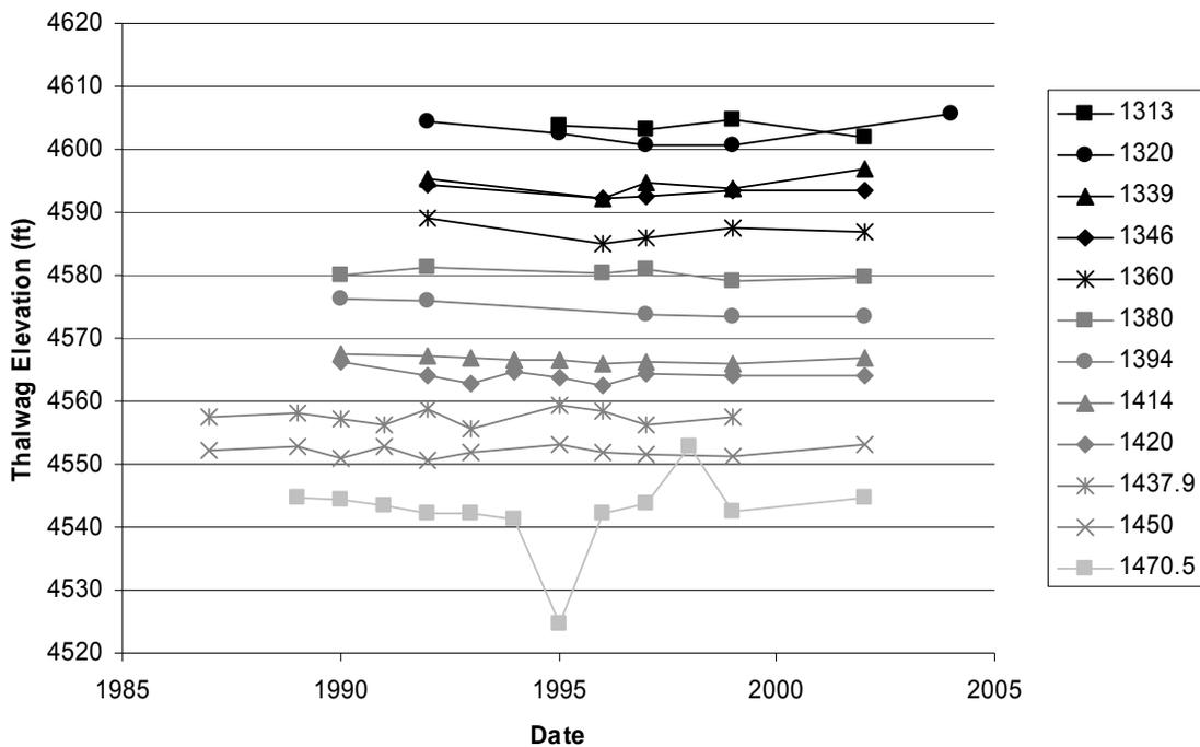
**Figure 3.5 Change in thalweg elevation by SO-line**
