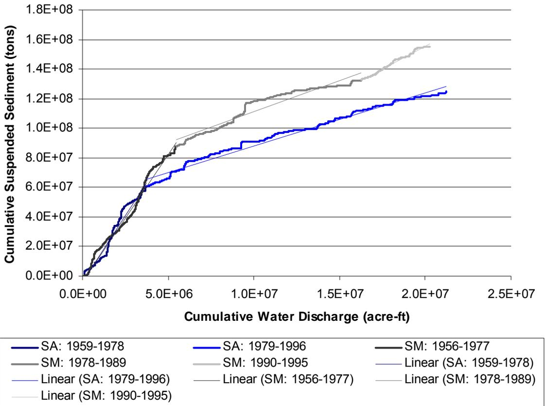
**Figure 4.3 Suspended Sediment Concentration Double Mass Curve**
