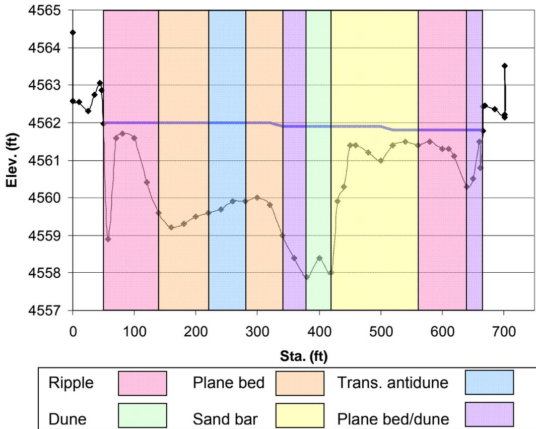
Figure 6.7 Typical cross-section with bedforms
