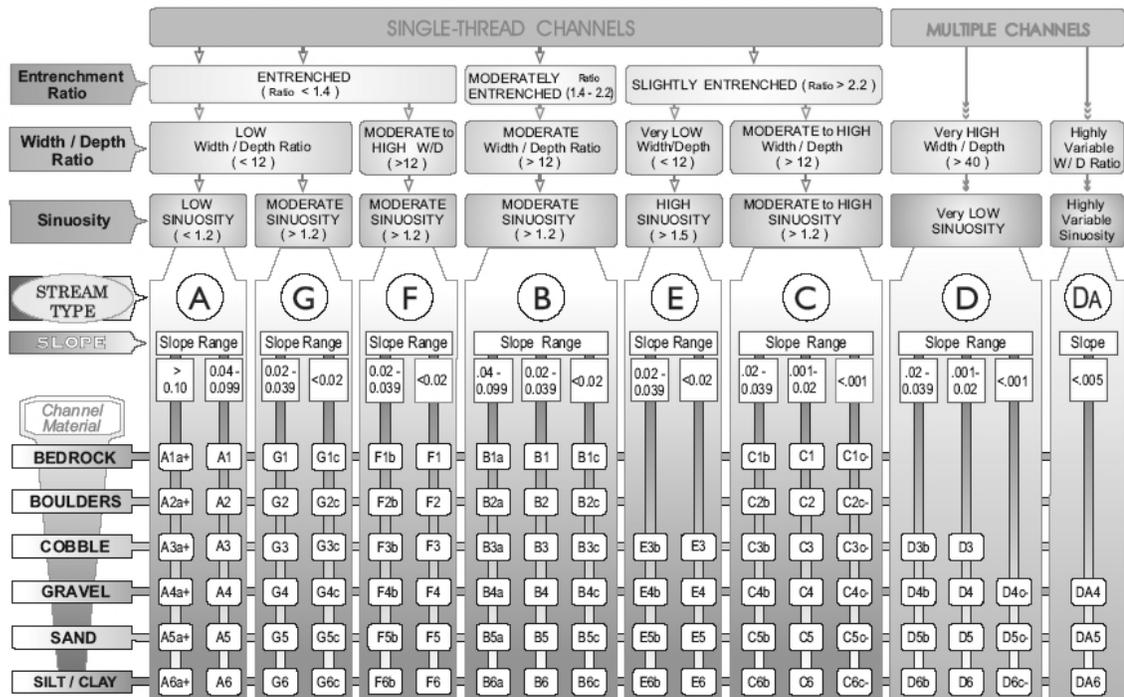
KEY to the ROSGEN CLASSIFICATION of NATURAL RIVERS. As a function of the "continuum of physical variables" within stream reaches, values of Entrenchment and Sinuosity ratios can vary by +/- 0.2 units; while values for Width/Depth ratios can vary by +/- 2.0 units.
