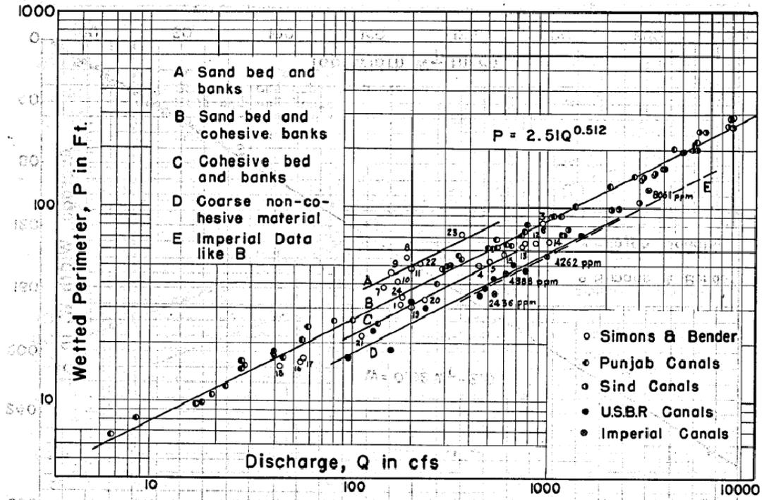
Figure 7.1 Variation of wetted perimeter P with discharge Q and type of channel (after Simons and Albertson 1963)
