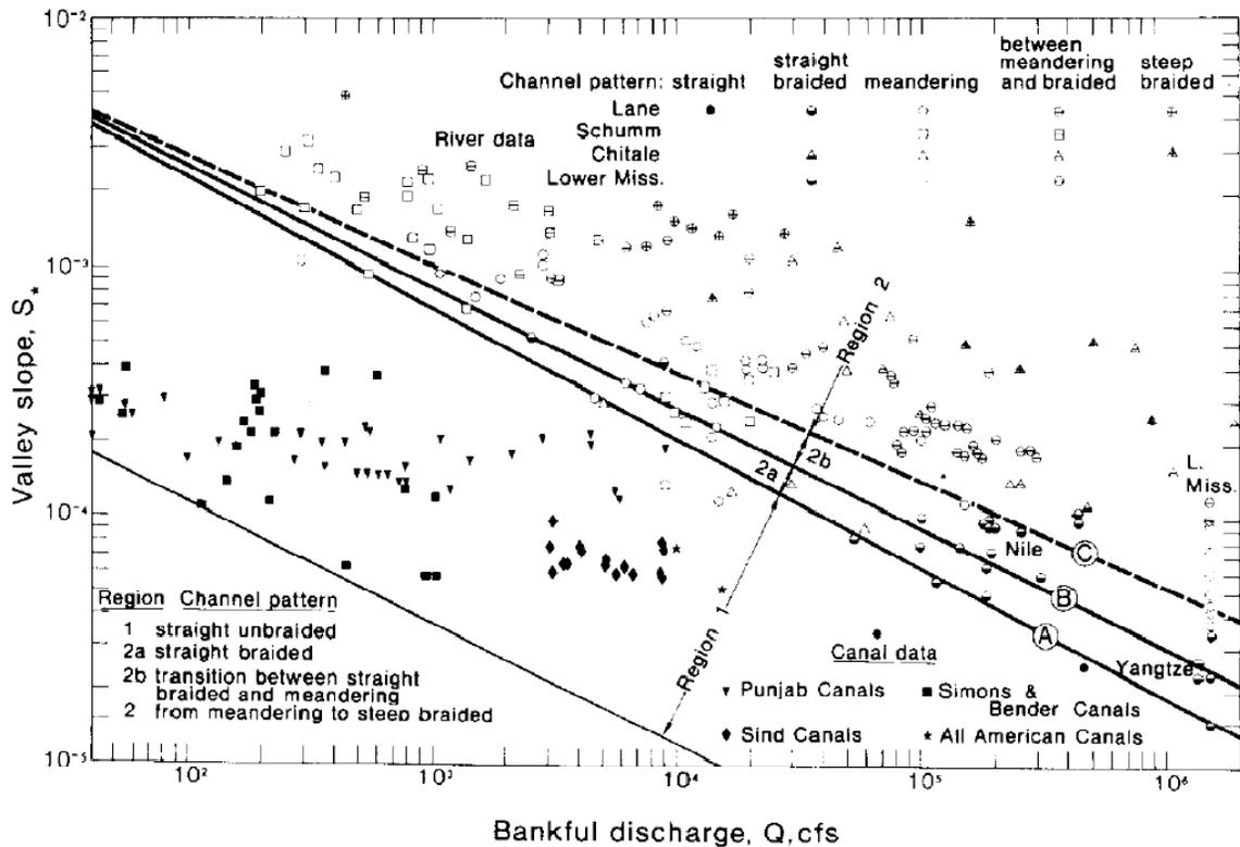
Figure 3.2 Chang's Stream Classification Method Diagram (Chang 1979)
