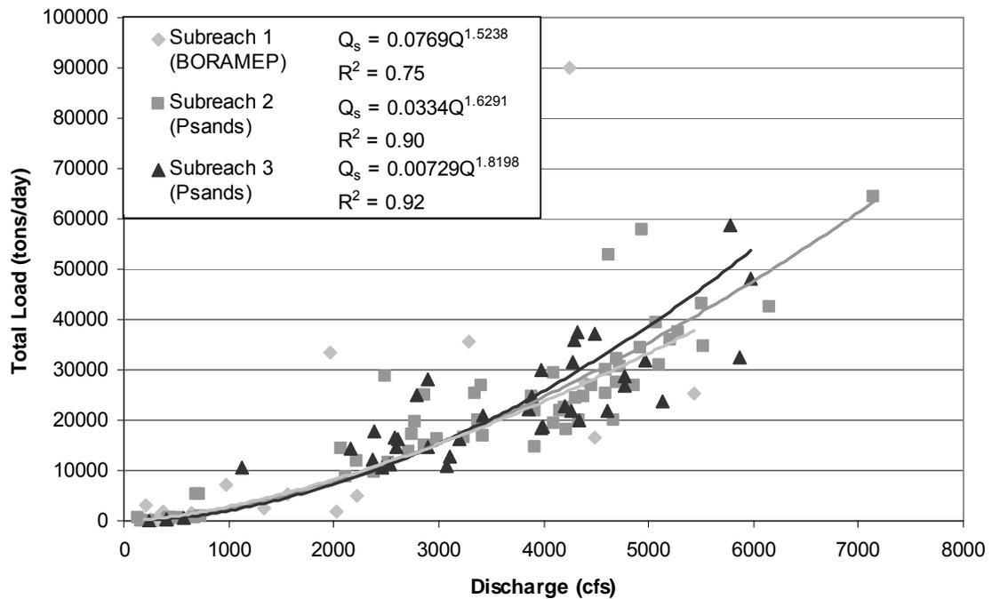
Figure 7.8 Total load rating curves from BORAMEP and Psands
