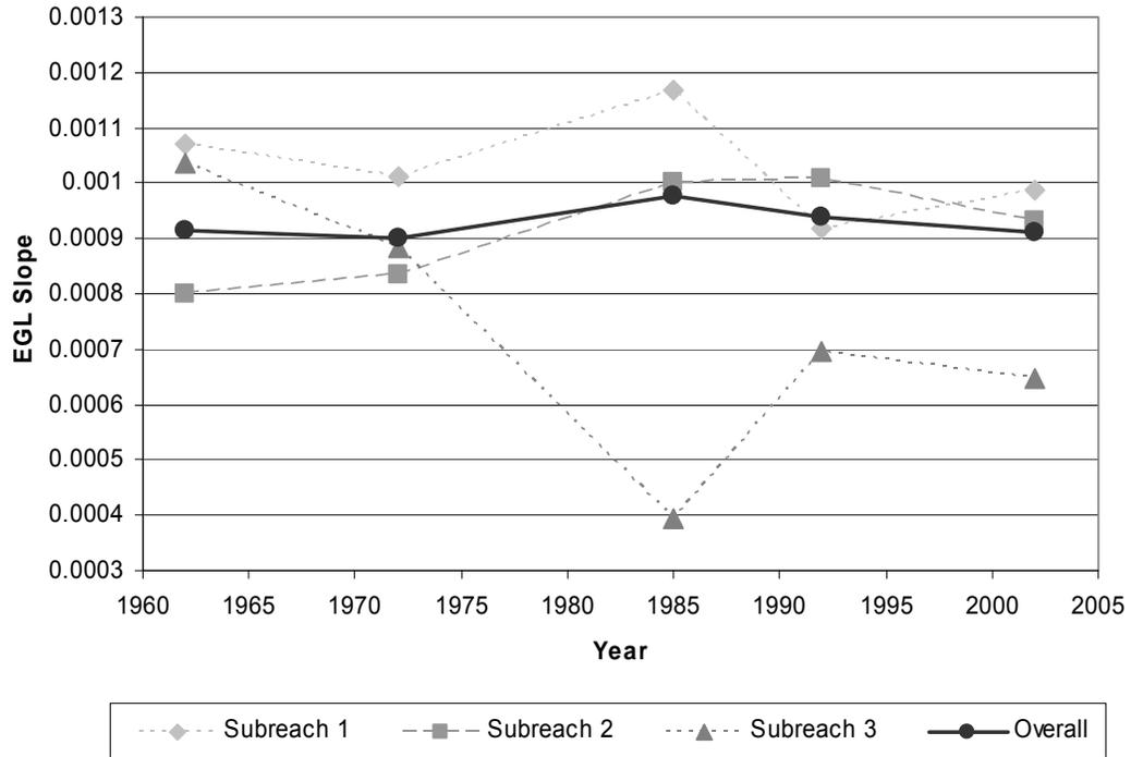
**Figure 3.9 Energy grade line slope**
