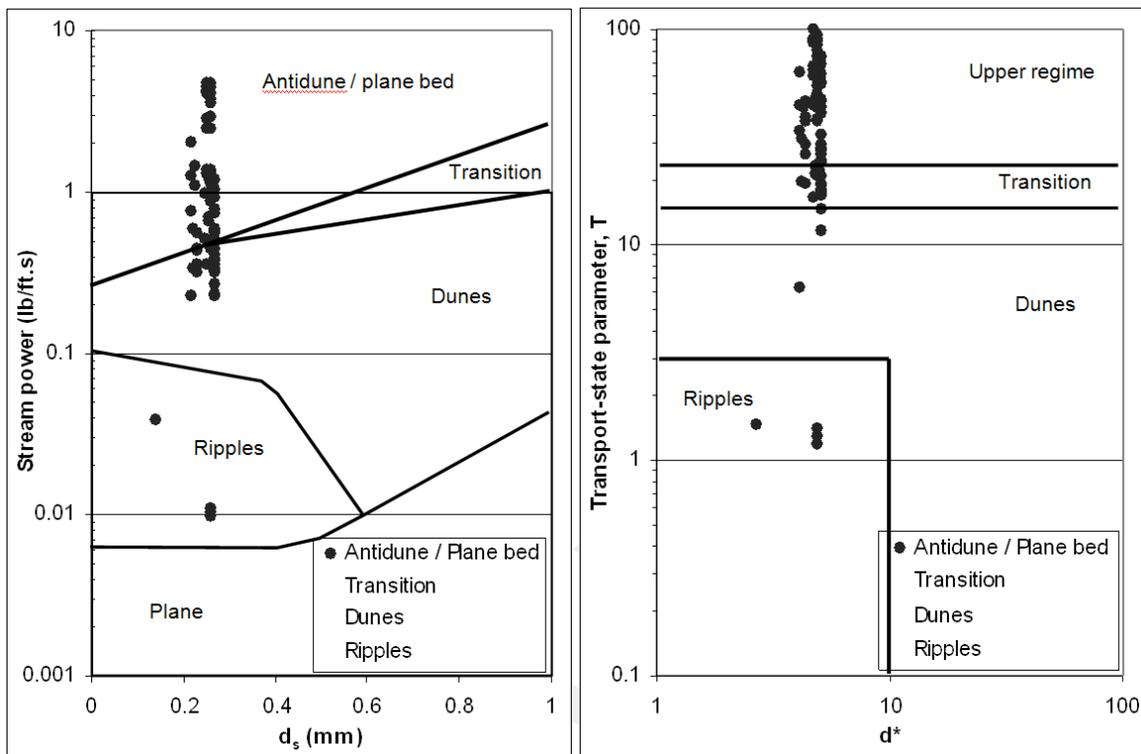
Figure 6.6 Observed antidunes/plane bed plotted on graph from Simons and Richardson (L) and van Rijn (R) (after Julien 1998)
