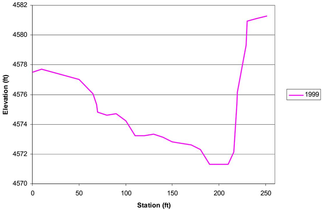
**Figure A.16 Cross-section survey at SO-line 1398**
