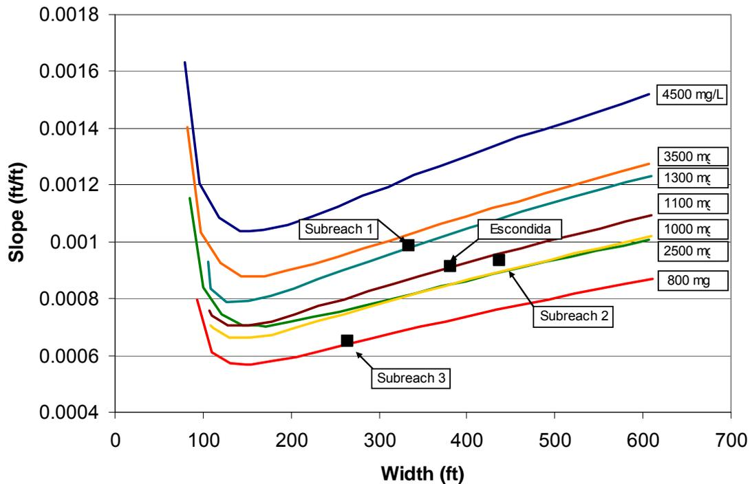
Figure 7.9 Results from SAM for 2002 conditions at Q = 5000 cfs
