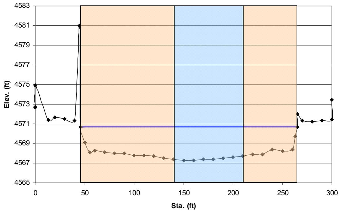
Figure E.6 Cross-section 1414 (surveyed 5/23/1992, Q = 3800 cfs)
