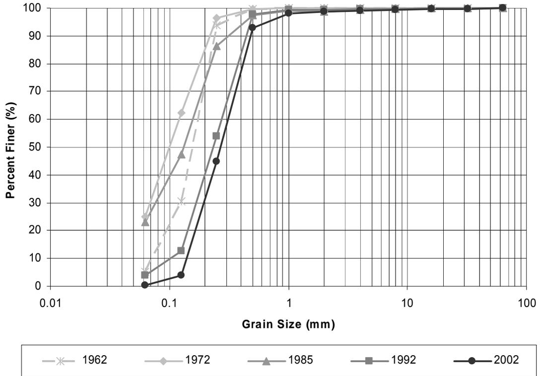
Figure 3.17 Bed material particle size distributions
