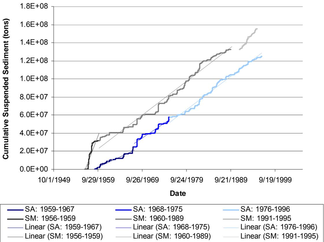
**Figure 4.2 Suspended Sediment Discharge Single Mass Curve**
