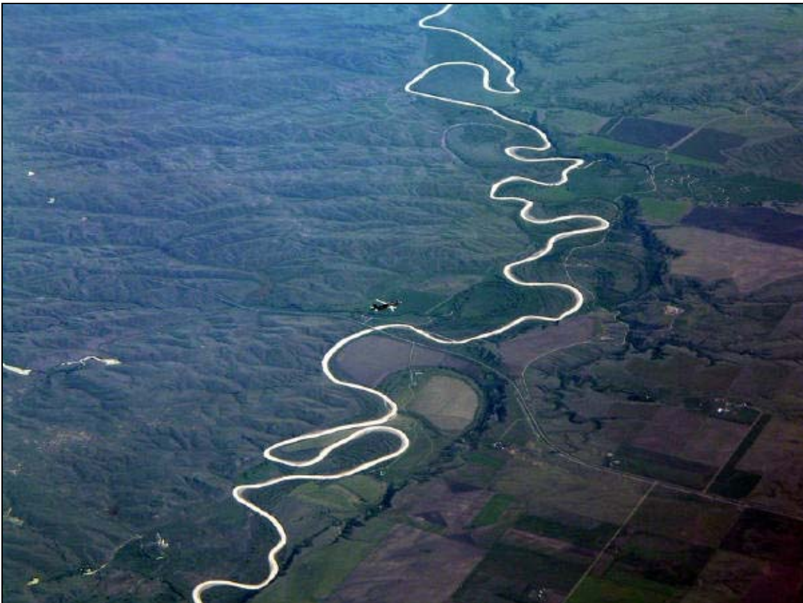
Figure 15: Evidence of channel migration in the Mississippi River. Source: U.S. Geological Survey
