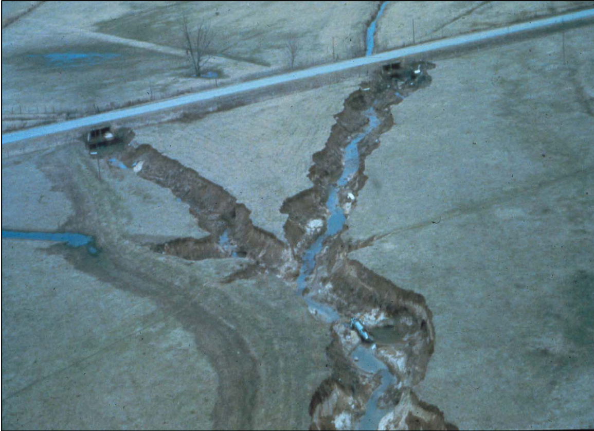
Figure 11: Headcutting in the lower Mississippi River. Source: U.S. Army Corps of Engineers
