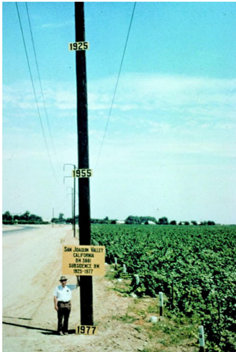
Figure 2 From the UNESCO Guidebook, Land Subsidence "Joseph F. Poland of U.S. Geological Survey stands near bench mark S661 southwest of Mendota in the San Joaquin Valley, California. The bench mark site subsided 9m from 1925 to 1977, because of intensive withdrawal of ground water. Signs on the power pole indicate the respective positions of the land surface in 1925, 1955, and 1977." (Poland, 1984)
