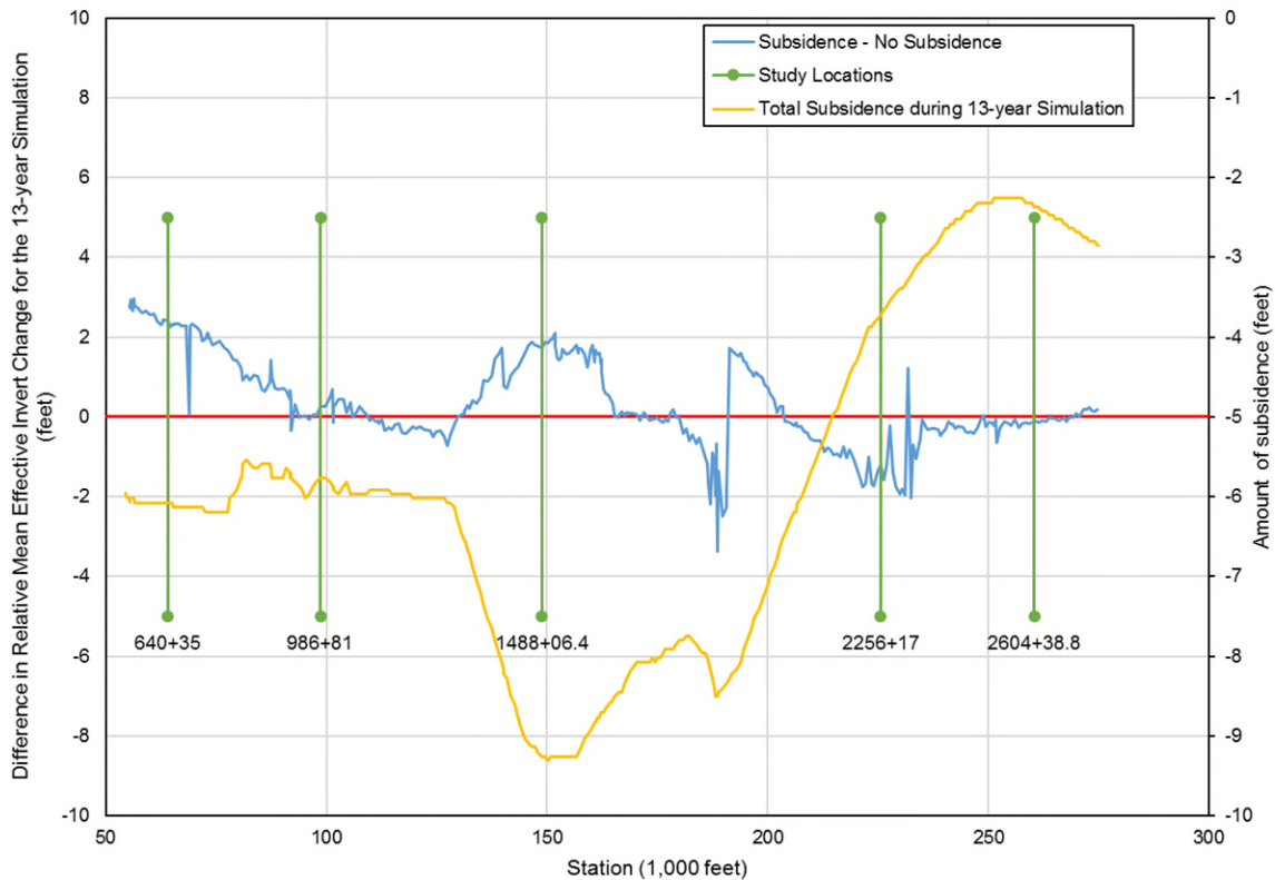
Figure 37 Difference in the Relative Mean Effective Invert Change in feet for the duration of the 13-year simulation for the No Subsidence, and Subsidence models.
