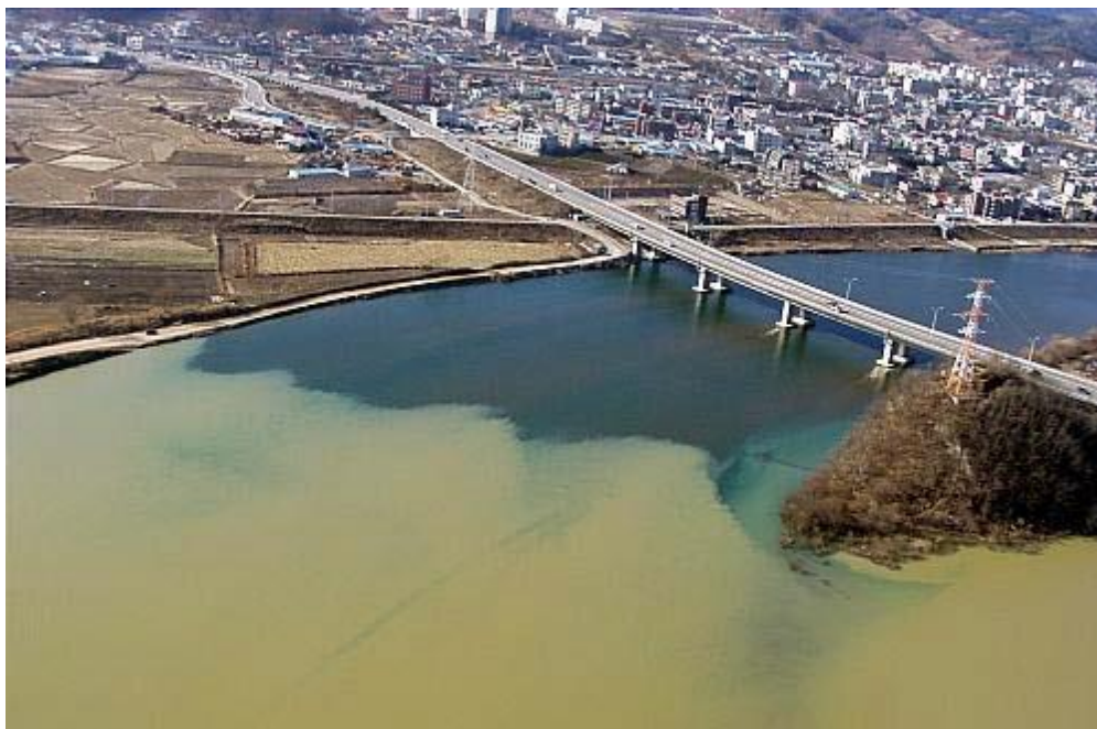
Figure 14: Discharge of highly turbid water during Typhoon Ewiniar downstream of Soyang Reservoir in 2006 (An, 2012)
