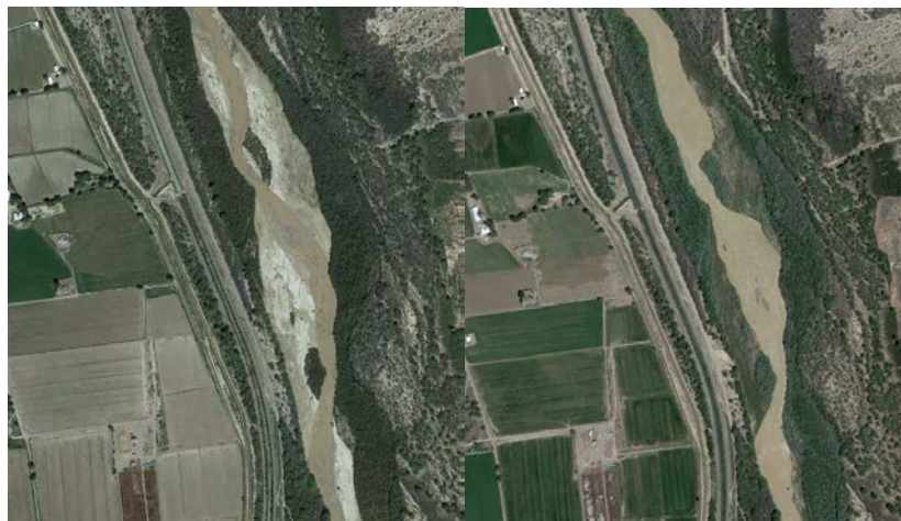
Figure 39 Subreach SA3 from October 2013 to April 2017 showing vegetation encroachment and narrowing in the main channel. Flow direction is from top to bottom, discharges unknown. Imagery from Google Earth
