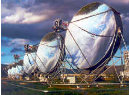
Figure A-10 SOLO/SBP Stirling Solar Systems at the Plataforma Solar de Almería
