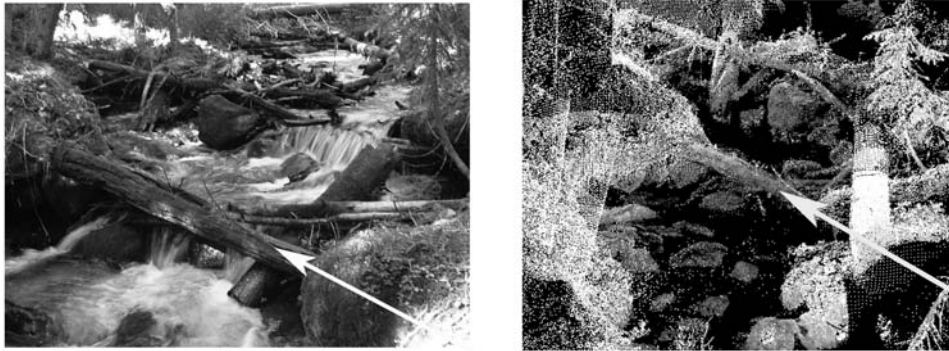
Figure 3. Example of the results of a LIDAR scan of ESL9. The arrow is pointing to the same log on (left) the photograph and (right) the point cloud. The photograph and scan image are both showing a wood step in ESL9.
