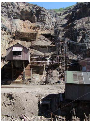
(Above: Waste rock pile 14 and the Tramway tributary area in Belden: a key source of zinc loading to the Eagle River.)
