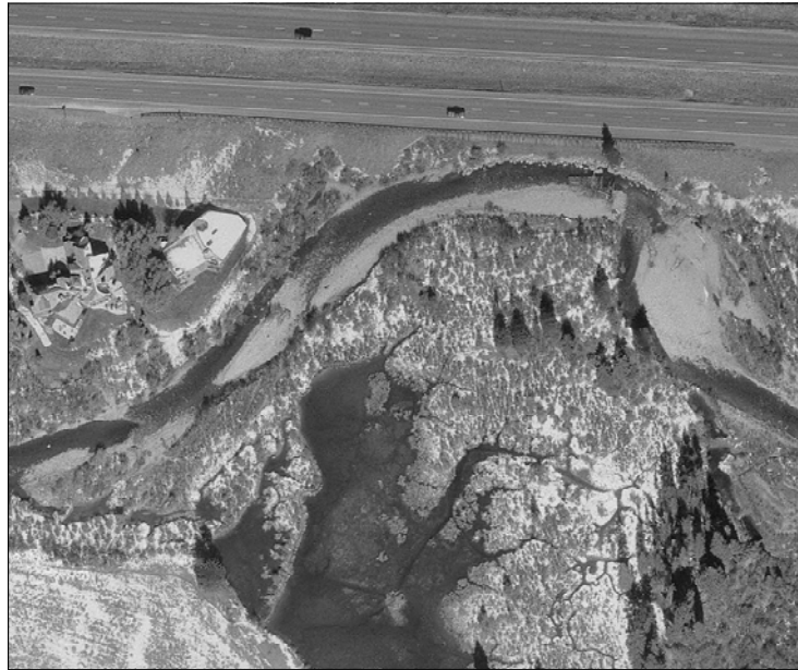
Figure 4.137: Bar formation and aggradation along Gore Creek near East Vail.
