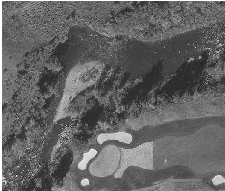
Figure 4.117: Chute cutoff at Arrowhead golf course.
