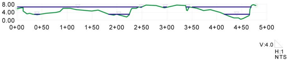
Figure 11: Section 4 at low and high flow, left descending bank on left. Low flow calibrated to survey date, high flow taken from high water marks. Note old point bar by station 3+50, now being dissected, divided reach, near vertical bank profile against right bank, and twin side channels.
