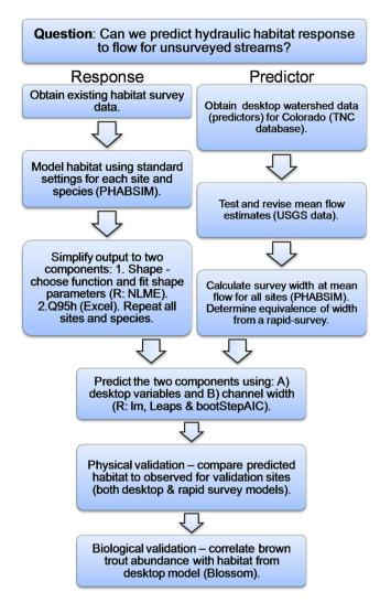
Figure 1. Flow chart summarizing our methods. The name of data analysis software is given in parentheses, including the name of packages implemented using R Project software. TNC, The Nature Conservancy; PHABSIM, Physical Habitat Simulation; NLME, nonlinear mixed effects
